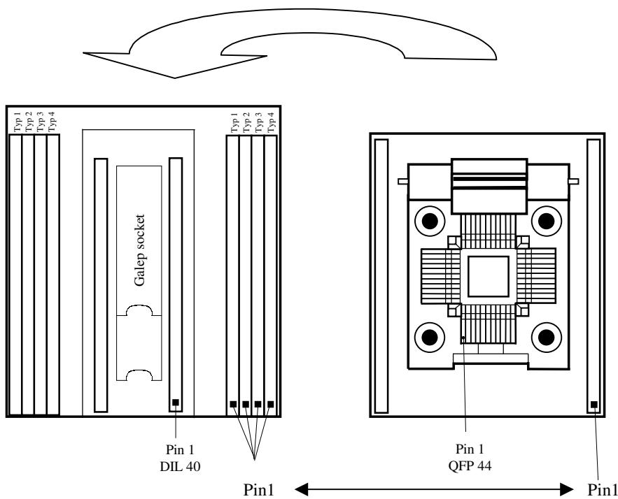
Please carefully note the correct orientation, when inserting the upper board into the lower board (see diagram above). The diagram also illustrates how the adapter will fit into the GALEP.
